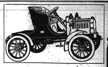
Drive: Through propeller shaft and bevel gears (running in oil and enclosed in dust-proof cases), such as is used on the Pierce \$5,000 car, the Packard \$4,000, the Peerless \$5,000, National \$3,000, Austin \$4,500, Roval \$3,500, etc. 60 per cent. of ALL American makers and 85 per cent. of the makers of high-priced cars are using shaft drives on their 1906 cars. No chains whatever on the Maxwell.
